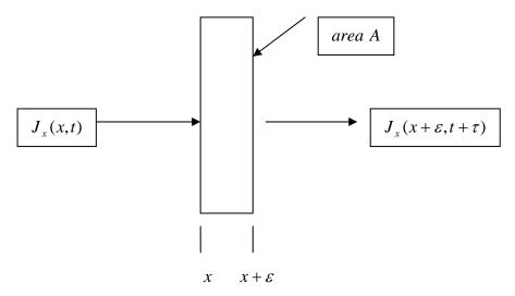
Consider the box in the figure. In a period of time  $\tau$ ,  $J_x(x)A\tau$  elements will enter from the left and  $J_x(x+\varepsilon)A\tau$  elements will leave from the right. The volume of the box is  $A\varepsilon$ . If the elements are neither created nor destroyed, the number of elements per unit volume in the box must increase at the rate
