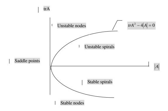
By the Poincare-Bendixson theorem, limit cycle solutions exist if  $(u_0, w_0)$  is an unstable spiral or node, but not if it is a saddle point. For an unstable node or spiral to occur, we require
